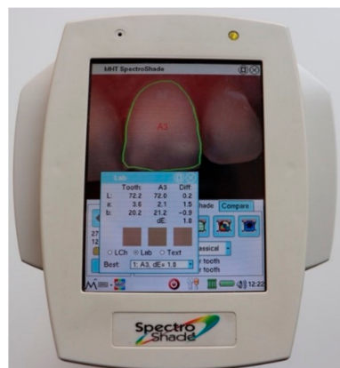
Figure 1. Defining the tooth area and the measurement of CIE L*a*b* values by the spectrophotometer.
