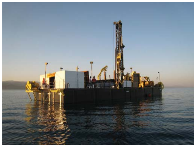
Figure 7. The new large Deep Lake Drilling System (DLDS) operated by DOSECC with the new top-head-drive rotary rig.
