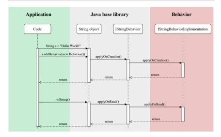
Figure 11.1: Message flow between software components
