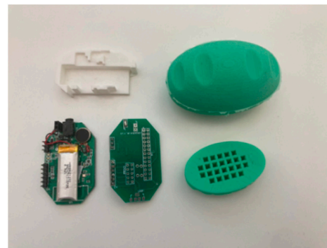
Figure 3. Smart Sensor Egg. The device is about 60 mm tall and weighs 50 g. (Left side): electronic board with an integrated pressure sensor and accelerometer. (Right side): silicone cover.
