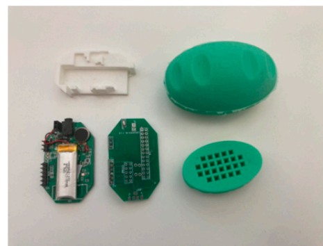
Figure 3. Smart Sensor Egg. The device is about 60 mm tall and weighs 50 g. ( Left side ): electronic board with an integrated pressure sensor and accelerometer. ( Right side ): silicone cover.
