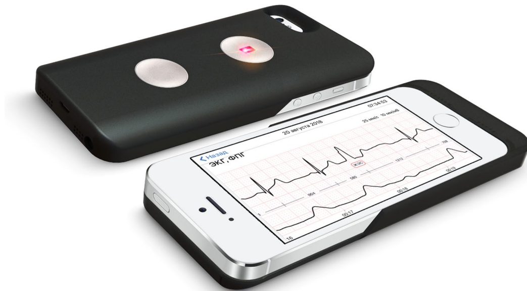
Figure 2. Single-channel electrocardiograph “CardioQVARK®.”
