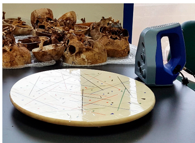
Figure 1. The Artec Space Spider scanner, the rotating table used to perform the scans and selected specimens.
