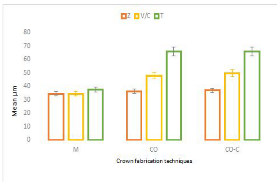
Figure 2: Marginal discrepancy values ( \mu\text{m} ) for monolithic(M), CAD-on technique (CO); CAD-on cemented technique (CO-C) at zirconia stage (Z); after porcelain veneering and cementation (V/C) and after thermomechanical fatigue (T)
