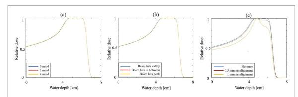
**Figure 9.** Analysis of the robustness of the RF under possible errors and misalignments for a 100 MeV beam. (a) The beam hits the RF with 0, 2 and 4 mrad angle to the normal of the RF's surface. (b) The beam's center is on the valley, on the peak or on a position between the two. (c) The M-RF is not aligned with the N-RF, we consider 0.05 and 0.1 cm misalignment.
