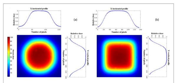
**Figure 7.** Dose profile perpendicular to the beam direction with the RF. (a) Sphere of 2 cm radius measured at 17 cm depth. (b) Box of 4 cm lateral size measured at 16 cm depth.
