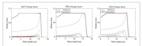
**Figure 6.** 12 cm (4–16 cm) SOBP generated with and without RF is compared. (a) SOBP created without RF with 53 energy layers (1.5 MeV energy steps). (b) SOBP generated with the RF in the configuration of the M- and N-RFs being aligned. (c) SOBP achieved by combining the maximum and minimum broadening depth dose curves. In (b) and (c) the simulated curve is benchmarked with the measured data.
