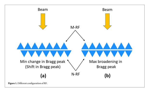
The displacement between the RFs can be varied continuously between the extremes shown in figure 1(a) and figure 1(b), respectively; thereby moving the two ridges relative to each other, any possible broadening between minimum and maximum can be obtained, as desired for the treatment.
