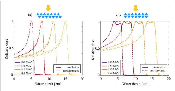
Figure 5. Comparison between measurements (dot line) and TOPAS simulations (full line). The RF is positioned in the minimum (a) and maximum (b) broadening configuration.
