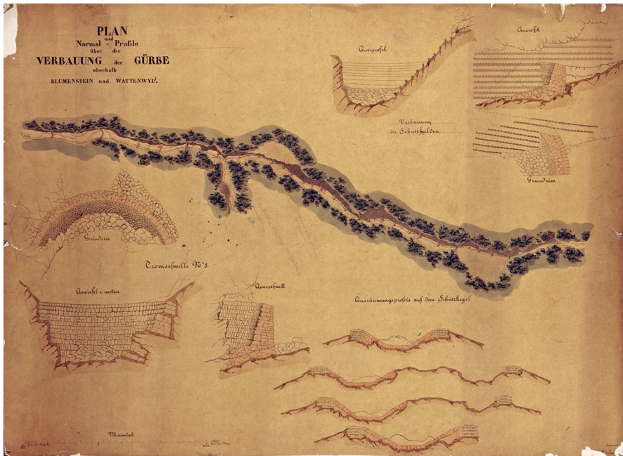
Fig. 4 Overall plan and profiles for the construction of the check dams in the gorge of the Gürbe River, ca. 1860. State archive of the Canton of Bern, StAB AA V 116b
