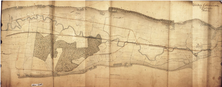
Fig. 3 Map of the Gürbe River between Toffen and Belp, 1870. The map shows the old meandering course of the river and the new straight channel. State archive of the Canton of Bern, StAB AA V 130
