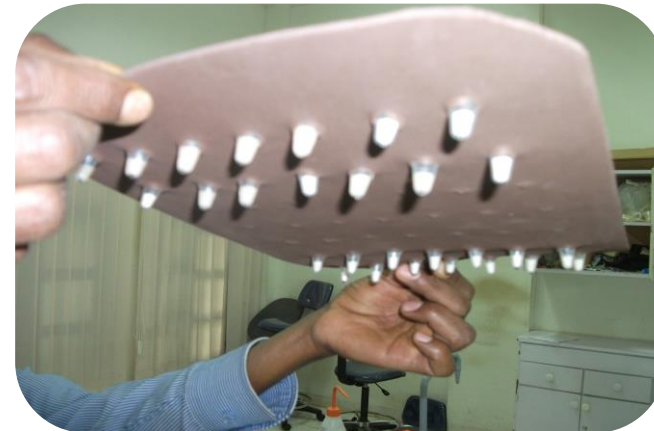
(E) Silica sand support in holed tubes
