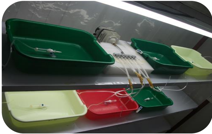
(A) -Aeration system installation using infusion set
