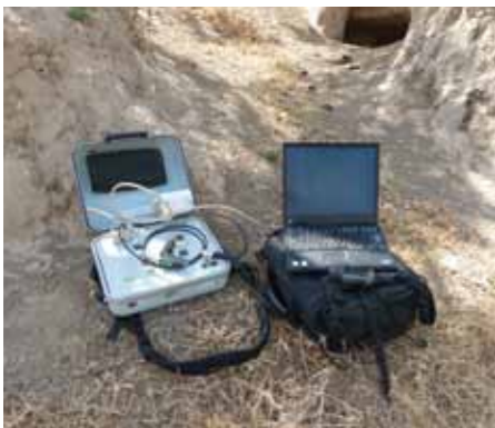
Modern field spectrometers are portable and can be operated by one person. Photo (Tajikistan): Christian Hergarten
