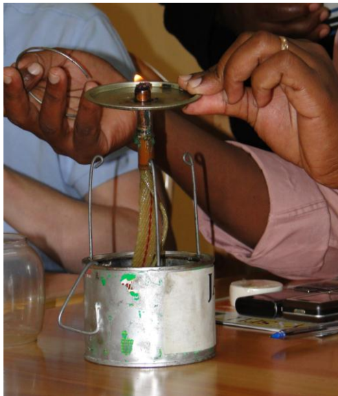
Figure 3: Jatropha oil lamp manufactured from an old tin. A copper tube has to be used to conduct the heat from the flame into the oil reservoir, in order to reduce the oil's viscosity (Photo. Ehrensperger 2011, Arusha, Tanzania)
