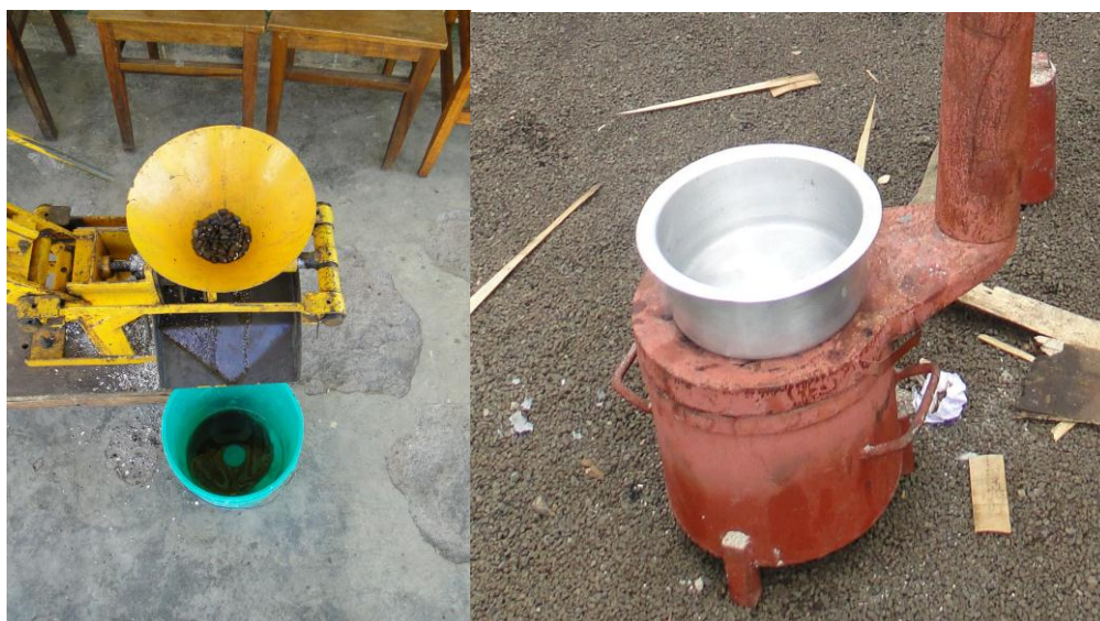
Figure 2: Left: Ram-press for extraction of jatropha oil from seeds. Right: Improved jatropha curcas seed-cake stove of Jatropha Products Tanzania Ltd. (JPTL). (Photos: Ehrensperger 2011, Arusha, Tanzania)
