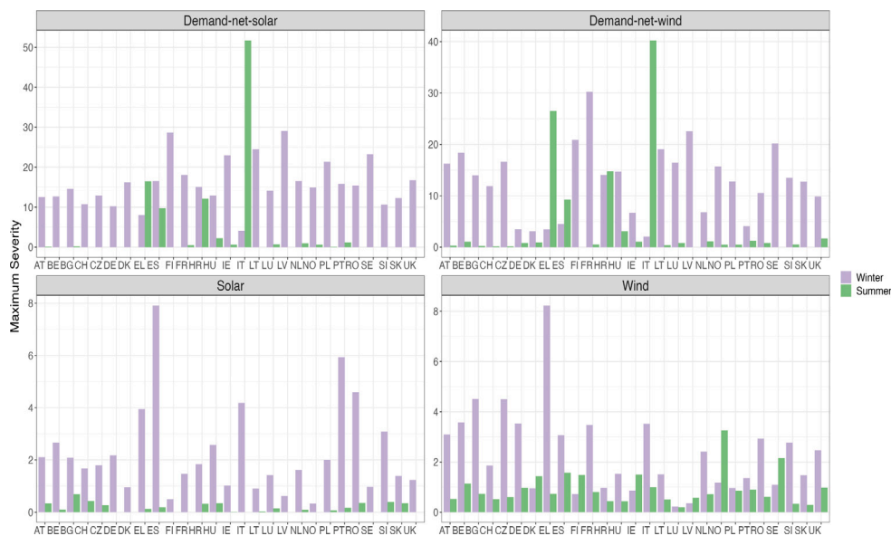
Fig. 6. Severity of energy droughts of individual sources: demand-net-wind and wind power, and demand-net-solar calculated for the summer and winter during the period of study 1979–2019 for each country. The long names of the countries acronyms are displayed in table S1. Please note the change of the scales due to the large variability between the demand-net quantities and the production.
