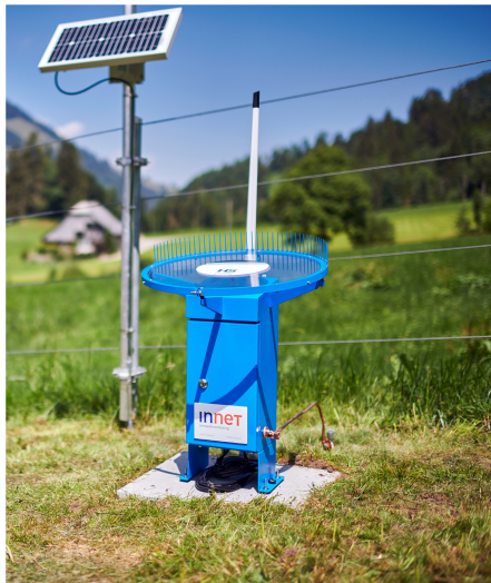
Figure 2. Left: An automatic hail sensor installed in the project 'Swiss Hail Network' (© Manu Friederich). Right: Zoom on the sensor Makrolon disc as a golf ball is falling (La Mobilière/Sascha Moetsch).
