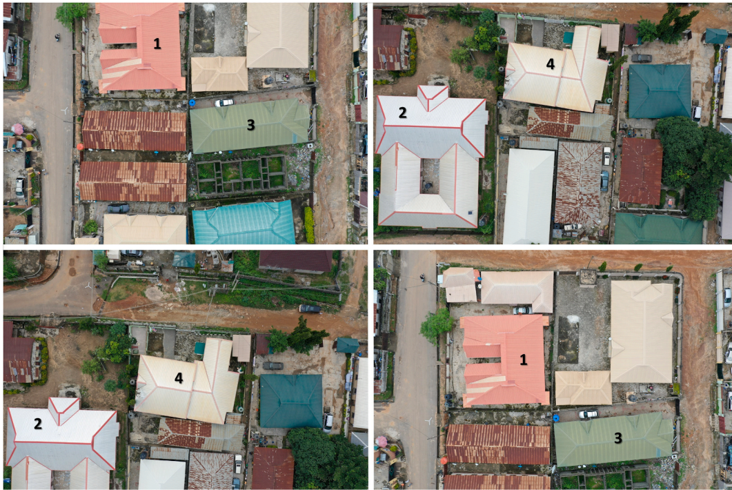
Fig. 4. A view of some of the UAV-acquired images showing feature overlap between adjacent images. The same features are numbered identically.
