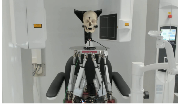
Figure 9: The skull is placed on top of the hexapod, at the height of a real patient’s head. The platform moves during the acquisition, creating reproducible motion parameters.
