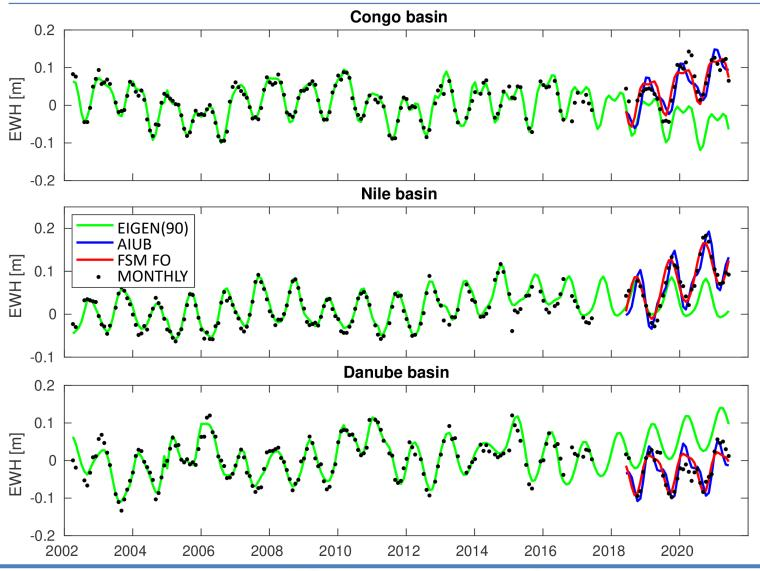
The time-series of monthly GRACE gravity field solutions was fitted in yearly batches for the EIGEN-GRGS-RL04 model.
