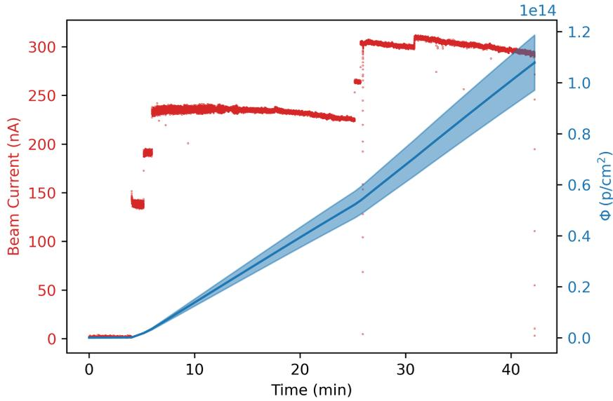
**Figure 9.** Observed beam current during an irradiation (red trace), together with the proton fluence delivered to the DUT (blue trace, the shaded area represents the 10% uncertainty on the fluence measurement). The steps in the beam current are due to the beam tuning performed by the cyclotron operator.
