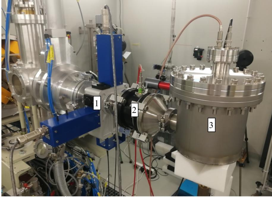
**Figure 10.** Validation of the irradiation setup. The UniBEaM (1) was installed before the collimator (2), mimicking a typical irradiation setup. A Faraday cup (3) was installed at the DUT position to measure the beam current.
