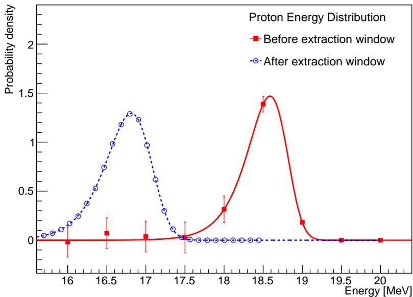
**Figure 8.** Distribution of the proton energy before and after extraction. The square points are the measured energy profile of the beam before extraction [23], fitted with a Verhulst function. The effect of a 300  $\mu\text{m}$  aluminium extraction window has been simulated and is shown by the circle markers.
