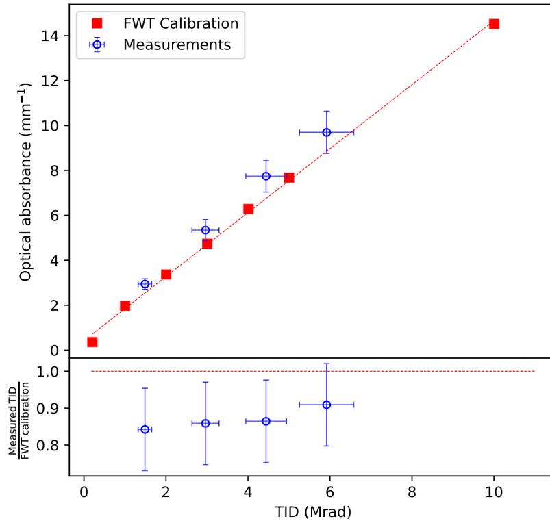
**Figure 12.** Comparison between the TID measured using the method described in this document (blue circles) and the one determined from the change in colour of the radiochromic films, according to the calibration provided by FWT (red squares) [30]. The two measurements are compatible within 15% as shown by the ratio in the bottom plot.
