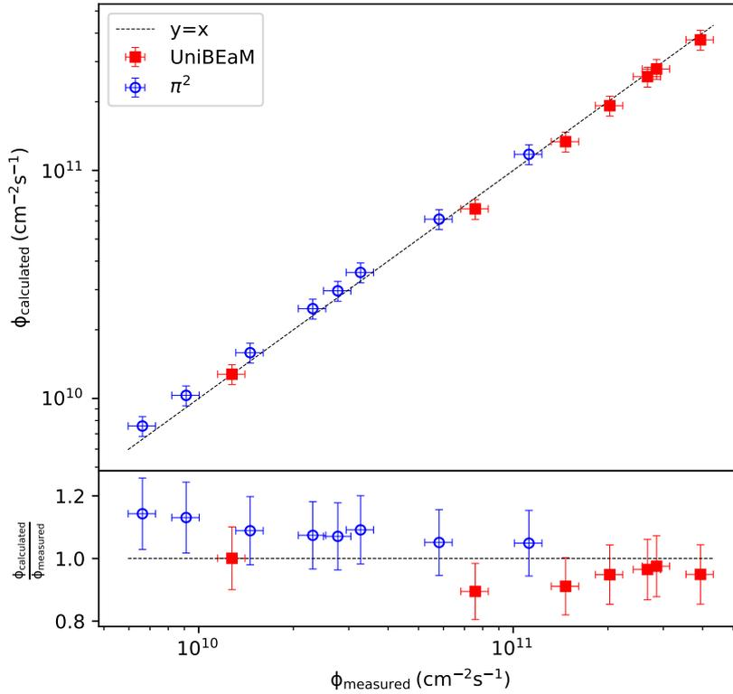
**Figure 11.** Proton flux obtained using Equation 3.2 for the UniBEaM (red squares) and the  $\pi^2$  (blue circles), as a function of the flux obtained from the beam current measured on the Faraday cup. To guide the eye, the dashed line represents the identity function. For both beam profilers, the calculated proton flux is compatible within 10% with the Faraday cup measurement, as shown by the ratio in the bottom plot.
