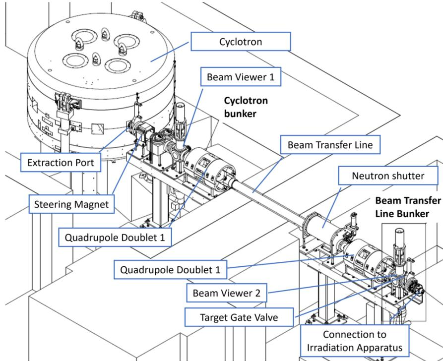
**Figure 2.** Scheme of the cyclotron and irradiation bunkers. The cyclotron bunker is separated by a 1.8-m thick concrete wall from the BTL bunker where the irradiation apparatus is located. This allows for easy access to the DUT shortly after irradiation, due to the low level of activity in the BTL bunker (below  $2 \mu\text{Sv h}^{-1}$ ).
