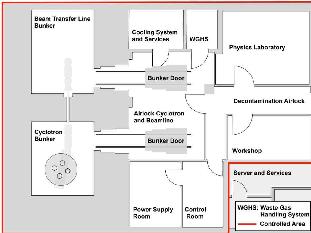
**Figure 1.** Layout of the cyclotron facility at the Bern Inselspital. It features two separate bunkers (depicted with their doors open in the figure) hosting the cyclotron and the BTL. In addition, a multi-purpose laboratory (Physics Laboratory) is available for post-irradiation studies.
