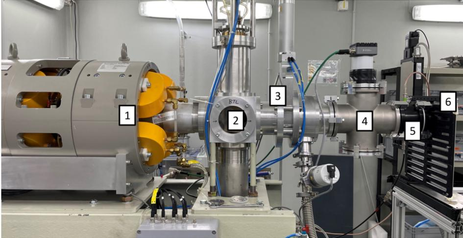
**Figure 3.** Irradiation setup. It consists of a quadrupole doublet (1), a beam viewer (2), the target vacuum valve (3), the two-dimensional beam profile monitor  $\pi^2$  (4) and the collimator terminated with an aluminium extraction window (5). The DUT is mounted and aligned on the remote controllable 2D stage (6).
