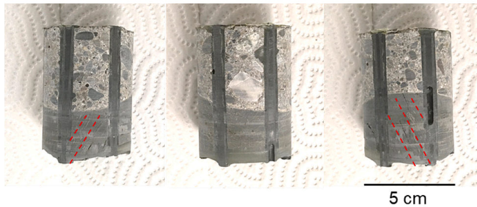
Fig. 1. Three sides of the core sample just after dry drilling: Concrete above, OPA (dark) below the oblique interface, dark vertical traces of intersected stabilisation pins. Dashed red lines visualise the bedding traces. (For interpretation of the references to colour in this figure legend, the reader is referred to the web version of this article.)
