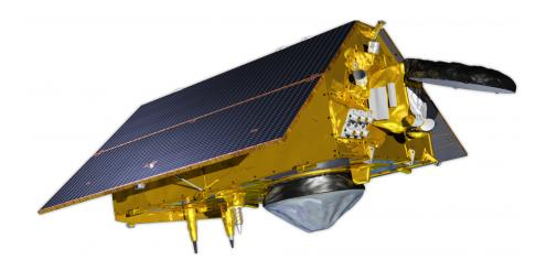
Figure 7: The altimetry satellite Sentinel-6 Michael Freilich. Flight direction (+x) is towards tilted microwave antenna on the right, +z downwards. Credits: NASA
