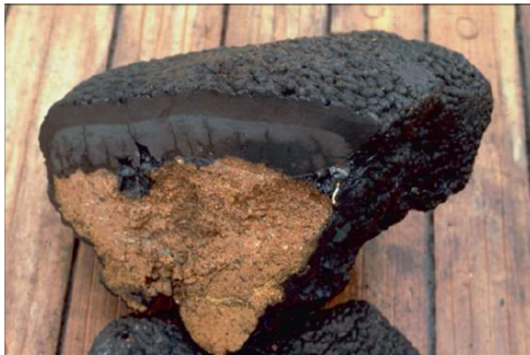
Fig. 3. Co-rich ferromanganese crust covering volcanic substrate rocks. The thickness of the crust is about 80 mm. Sample collected from a seamount in the Central Pacific Basin. Picture modified from (Halbach et al. 2017).
