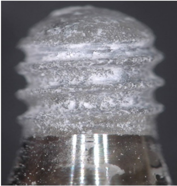
Fig. 4 Example of light optical microscopy image of a TL Ø4.1×4 mm implant following torque-out from the water based adhesive cement formulation, following a curing time of 15 min. Based on the appearance of the surface, the mode of failure is predominantly adhesive in nature
