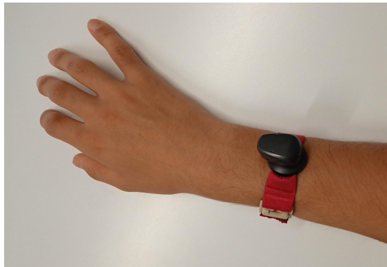
Figure 3. A bone conduction device (Cochlear Baha 6 max) used as a tactile aid just behind the wrist on a shortened softband.
