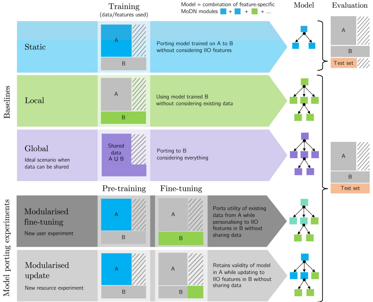
Fig 2. Experimental set up for porting MoDN modules in IIO settings. MoDN is tested in two “model porting experiments” (grey), where modules are ported from a larger source data set (A) for fine-tuning or updating on a smaller, imperfectly interoperable target data set (B). The two experiments represent either a scenario where a new user with different resources starts using a CDSS or where an existing user gains new resources and would like to merge training. Three baselines are proposed. Static (blue) where modules trained in A are directly tested in B, thus not considering additional IIO features. Local (green) where modules are only trained on the target data set B, thus without insights from the larger source data set. Global (purple) is the ideal but unlikely, scenario of when all data can be shared between A and B and the modules are trained on the union of data (A ∪ B). The modularised fine-tuning experiment, pre-trains on A and then fine-tunes all modules (for all features) on B (thus personalising the modules trained on A). The modularised update experiment, pre-trains the blue modules on A and then adds modules specific to the new IIO features (in green) which have been independently trained on B (thus preserving the validity of the modules trained on A). The colors of the MoDN modules illustrate their training on distinct data sets and their potential re-combination in the porting experiments. In particular, the modules trained on A (blue) and fine-tuned on B (green) are thus depicted in teal.
