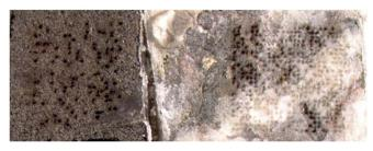
**Figure 2.** Photomicrograph of standard GSD-2G (left) and Boulder Creek Granite (right), showing ablation pits in both. The ablation pits, which define a rectangular grid of points separated by 0.2 mm, sample multiple mineral phases in the granite. The field of view is about 13 mm across. After these analyses were acquired, the sample mount was re-polished to flatness, and a new grid of points analyzed.
