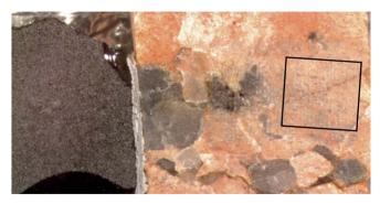
**Figure 7.** Photomicrograph of standard GSD-2G (left) and Pikes Peak Granite (right). Note that the ablation pits in GSD-2G are hard to identify, and can just be made out on the granite (square box; compare with Figure 2). The ablation pits define a rectangular grid of points separated by 0.2 mm. The field of view is about 13 mm across.
