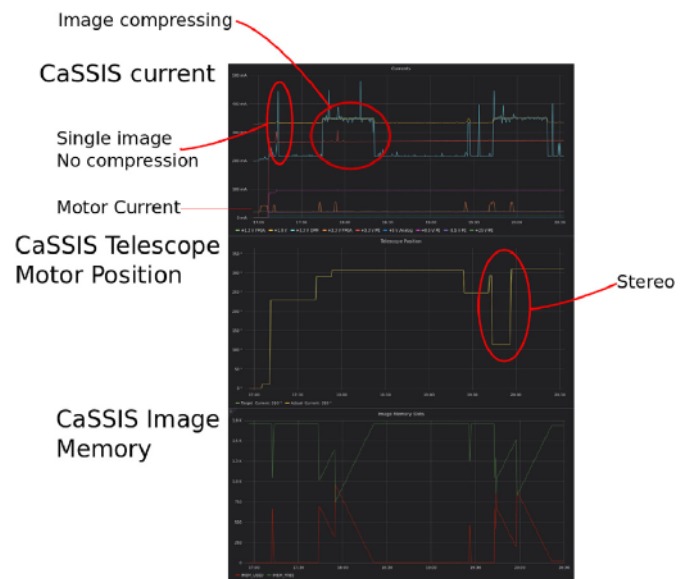
Fig. 7. CaSSIS Grafana panels: The telemetry can be checked live or as fast as it gets to the ground – it's of particular importance to monitor special occasions like a flight software update, but also allows for rapid reaction in case of instrument issues.
