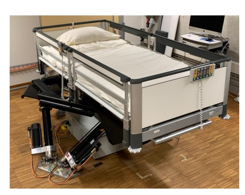
Cocktail of rotation (yaw, pitch, roll) at .25 Hz during sleep using a bed mounted on a 6 DoF motion platform.
