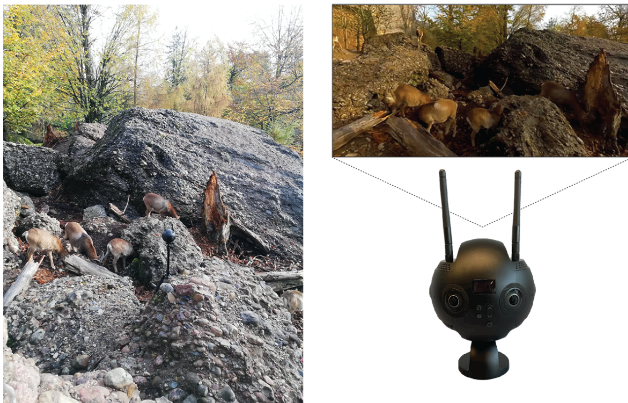
Figure 3. Camera setup and examples. (Left) Camera setup while filming on-location. (Top right) Screenshot of the final postprocessed video as it would be seen using the VR headset. (Bottom right) Insta360 Pro II camera (Arashi Vision Inc) showing the control panel. VR: virtual reality.
