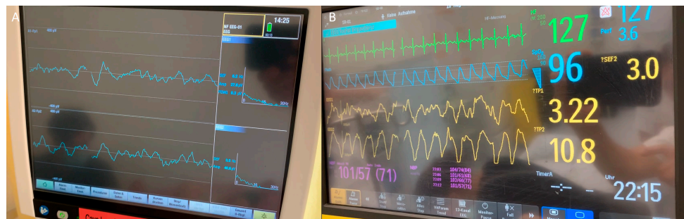
Figure A3. pocEEG tracings on a GE B450 Carescape monitor, normal activity (A) and on a Philips IntelliVue MX550 with seizure activity (B).
