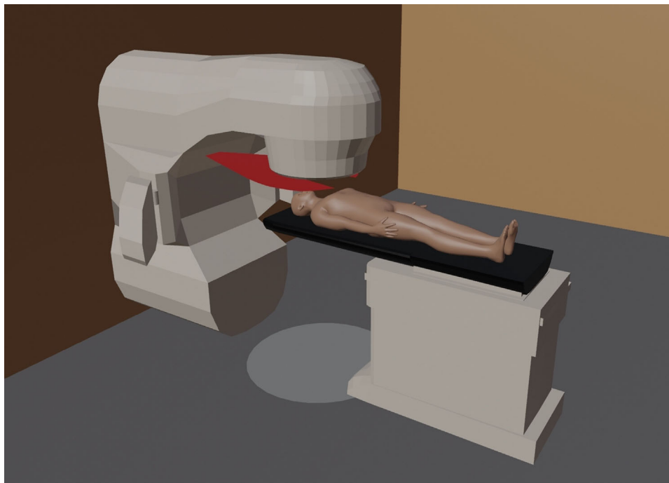
FIGURE 1 Screenshot of the Blender model including gantry and table stand in light grey, table top in black, laserguard in red and patient in skin color.
