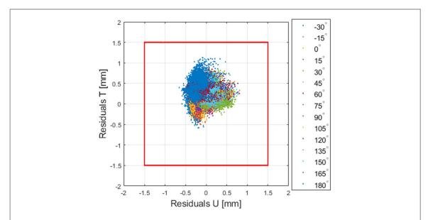
**Figure 6.** Beam position residuals measured in the nozzle and projected to iso-centre in transverse plane for ascending and descending energy sequences. Markers of the same colour show the measured positions at 17 different energies over the full scanning area of  $12 \times 20$  cm<sup>2</sup>. Measurements performed at different gantry angles are shown in different colours.
