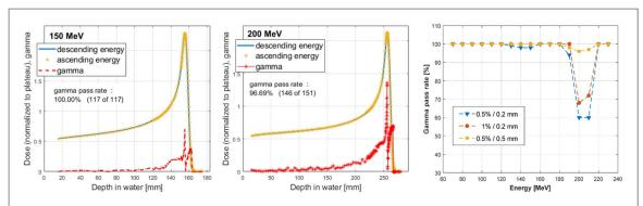
Figure 5. Left and centre: the integral depth dose curves for 150 and 200 MeV beams measured in both energy-changing directions: descending (blue solid line) and ascending (yellow star markers) and resulting gamma pass rate (red dashed line) for 0.5%/0.5 mm global gamma criteria. Right: gamma pass rate for different energies calculated using various global gamma criteria: 0.5%/0.2 mm—blue triangle markers, 1%/0.2 mm—red circle markers, 0.5%/0.5 mm—yellow square markers.
