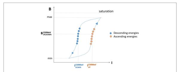
**Figure 2.** Schematic presentation of a hysteresis loop for a dipole magnet. Note, that B field is proportional to the particle momentum. Blue dots represent positions of energy layers within hysteresis cycle for descending and red dots for ascending energy directions (novel implementation).
