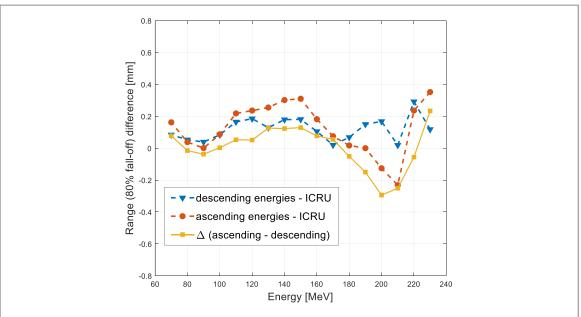
**Figure 4.** Proton range (80% fall-off) residuals between ICRU data and several data sets: descending energies (blue triangle markers), ascending energies (red circle markers) and range difference between beams acquired in opposite energy directions (yellow square markers).
