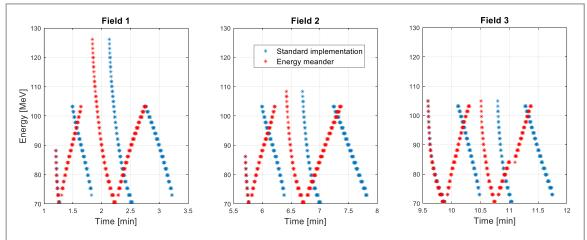
**Figure 10.** Energy as a function of time for the delivery of a 3-field clinical plan. Blue markers—energies delivered using one-directional energy changes. Red markers—plan delivery using energy meandering (novel technique).
