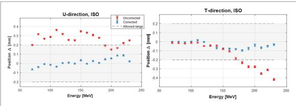
Figure 3. Positions residuals for Gantry 2 in T and U transverse directions before (red markers) and after (blue markers) the fine-tuning. The shaded area show the allowed range for position residuals.
