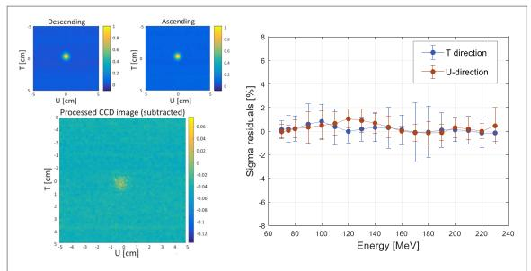
**Figure 7.** Left: the upper 2D profiles of 100 MeV beam applied using descending and ascending energy directions. The lower plot show the difference of two profiles shown above. Right: Beam sigma residuals (ascending—descending energies) in two transverse directions for ascending and descending energy sequences measured over the whole scanning and energy range in 10 MeV steps. The wiskers show the standard deviation for all measured values in a single energy layer.
