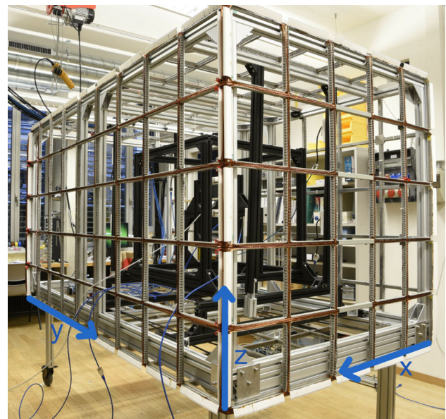
Fig. 5 Photo of the AMS prototype [17,18] mounted in the ETH laboratory. The smaller side of the frame, facing the window as seen on the photo, was kept open without windings – to allow easy access to the inside of the system
