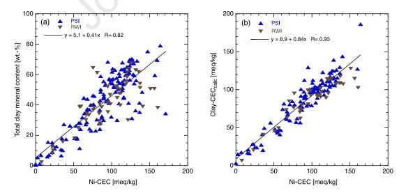
**Fig. 2.** Correlation of Ni-CEC with (a) total clay mineral content and (b) Clay-CEC<sub>calc</sub> for all rock samples from ZNO, NL and JO.
