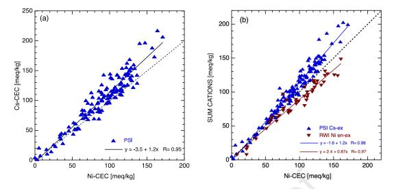
Fig. 3. Correlations of Ni-CEC with: (a) Cs-CEC and (b)  $\Sigma$ CATIONS obtained from Cs displacement experiments (blue symbols) and from Ni-en displacement experiments (brown symbols) for all samples from the three study areas. The dotted lines represent the one-to-one Cs-
