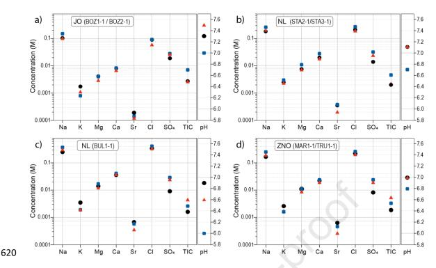
**Fig. 7.** Comparison of Opalinus Clay porewater compositions obtained from geochemical modelling (●: Model), squeezing (▲: SQ) and advective displacement (■: AD) for (a) JO (BOZ1-1/BOZ2-1), (b) NL (STA2-1/STA3-1), (c) NL (BUL1-1) and (d) ZNO (MAR1-1/TRU1-1).
