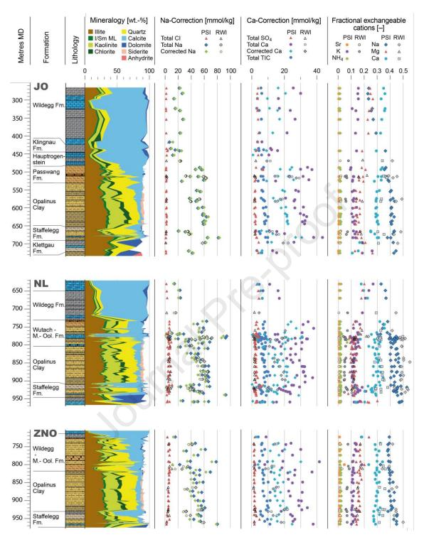
**Fig. 4.** Profiles of the study areas (JO, NL, ZNO) showing representative stratigraphic sections and the mineralogical data. The formation depths are adjusted to the profiles of BOZ1-1 (JO), STA2-1 (NL) and TRU1-1 (ZNO). The cation data includes results from Na-Correction method, Ca-Correction method and the fractional exchangeable cations Na, K, NH<sub>4</sub>, Mg, Ca, and Sr.
