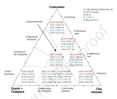
**Fig. 6.** Füchtbauer triangle (Füchtbauer, 1988) illustrating the values for 2:1 clay mineral content (illite + smectite + chlorite end-members), Ni-CEC, and fractional occupancy (average  $\pm$  stdv, number of samples) for all samples (PSI and RWI) of this study. Axes of total carbonate (top), quartz + feldspars (bottom left) and total clay (bottom right) contents are in wt.% and the lithological types 1–10 according to Füchtbauer (1988) are indicated.
