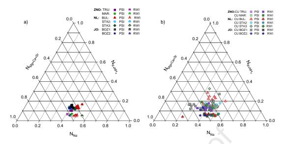
**Fig. 5.** Ternary representation of  $N_{Na}$ ,  $N_{K+NH4}$  and  $N_{Mg+Ca+Sr}$  determined for the samples from (a) Opalinus Clay and (b) the formations above and below the Opalinus Clay for ZNO, NL and JO.
