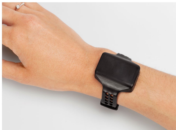
Figure 2. Cuff-less watch-like device used in the present study (PulseWatch, CSEM, Neuchâtel, Switzerland), which contains a photoplethysmographic (optical) sensor and an accelerometer, and can be attached at the wrist or the upper arm.
