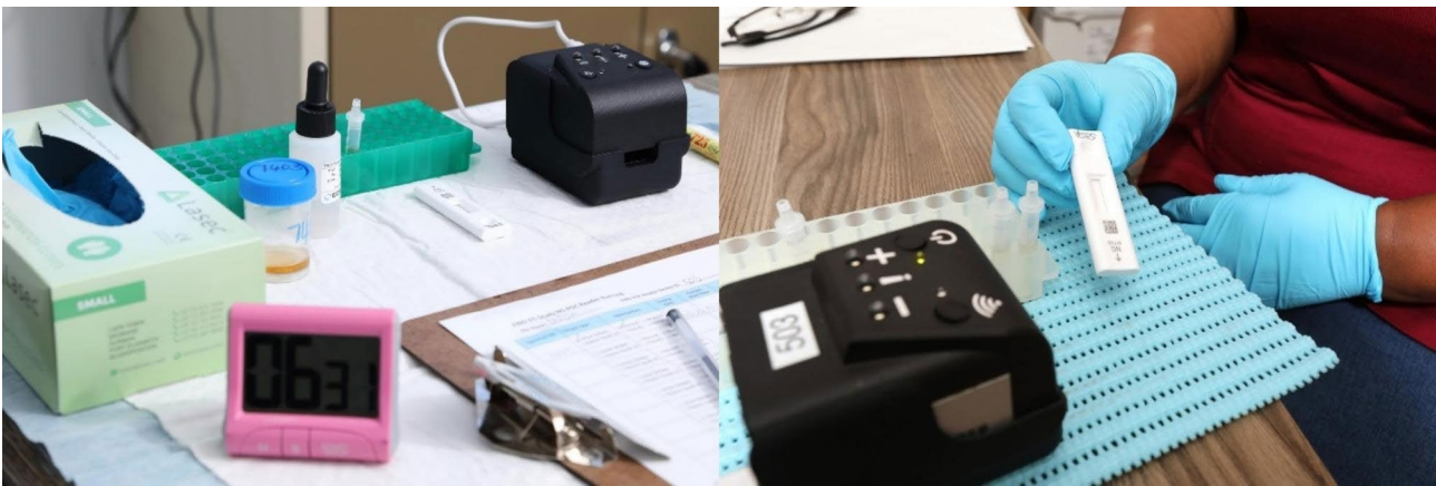
Fig. 2 NG-LFA device and testing set-up
