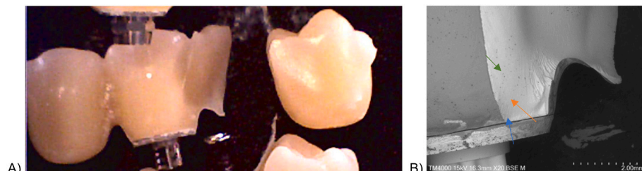
Fig. 3. A) Macroscopic and B) microscopic failure pattern showing origin (blue arrow), mirror (orange arrow) and mist (green arrow) area of fracture.
