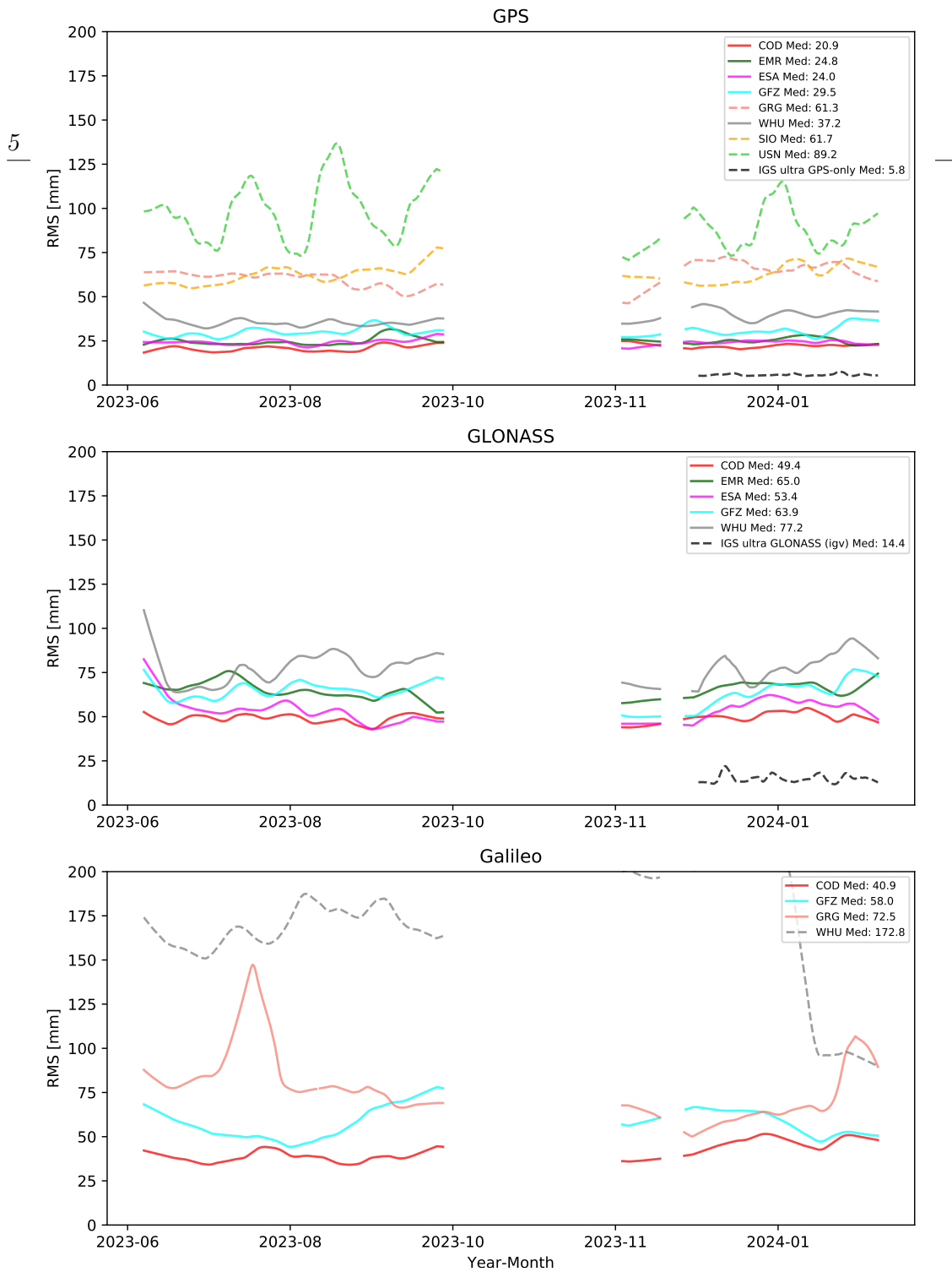
Figure 8: RMS of analysis center orbit solutions (smoothed) compared to the IGS combined orbits for the IGS multi-GNSS ultra-rapid demonstration products for GPS (top), GLONASS (middle) and GALILEO (bottom). The dashed lines are the AC solutions that are not weighted in the combinations, while the solid lines are the weighted ACs.
