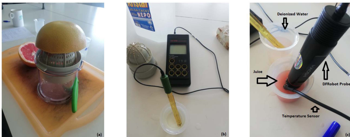
Figure 2. (a) The hand squeezing procedure. (b) Hanna pH meter. (c) DFRobot pH meter probe.
