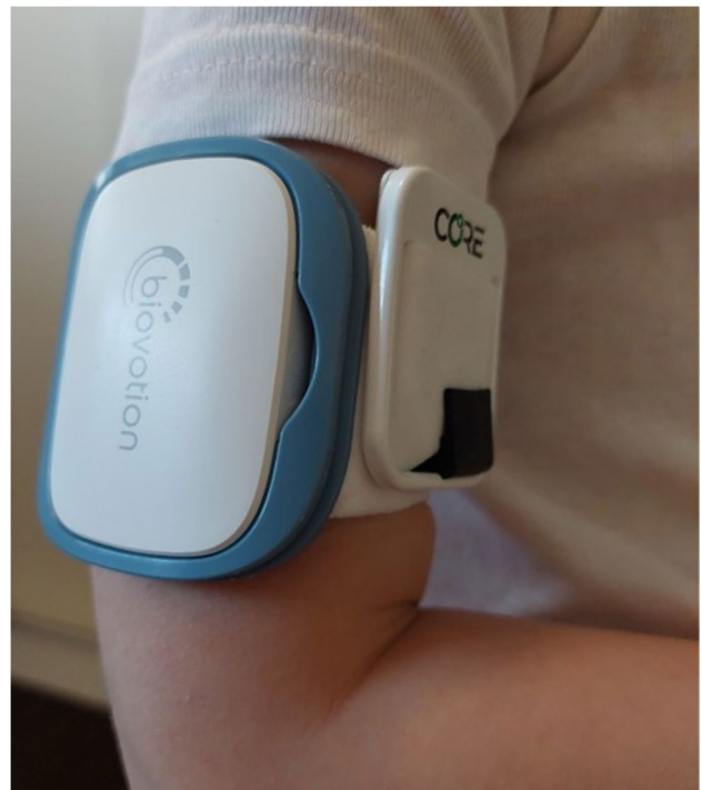
Fig. 1 CORE® and Everion® worn on the upper arm in a five-year-old child. Displayed are the Everion® (left) and the CORE® (right), both worn together on one armband on the right upper arm of a five-year-old child. The CORE® is secured with a small black clip, which prevents it from disattachment from the armband. Parents gave informed consent for the publication of this photography
