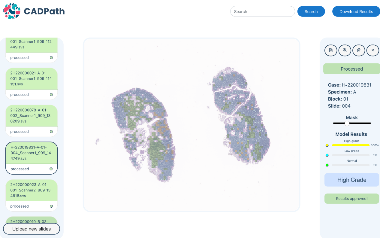
Fig. 9 | Main view of the CAD system prototype for CRS. Slide identification, confidence per class, diagnostic, mask overlay controller, results download as csv and slide search are some of the features visible. Slide identification is anonymised.
