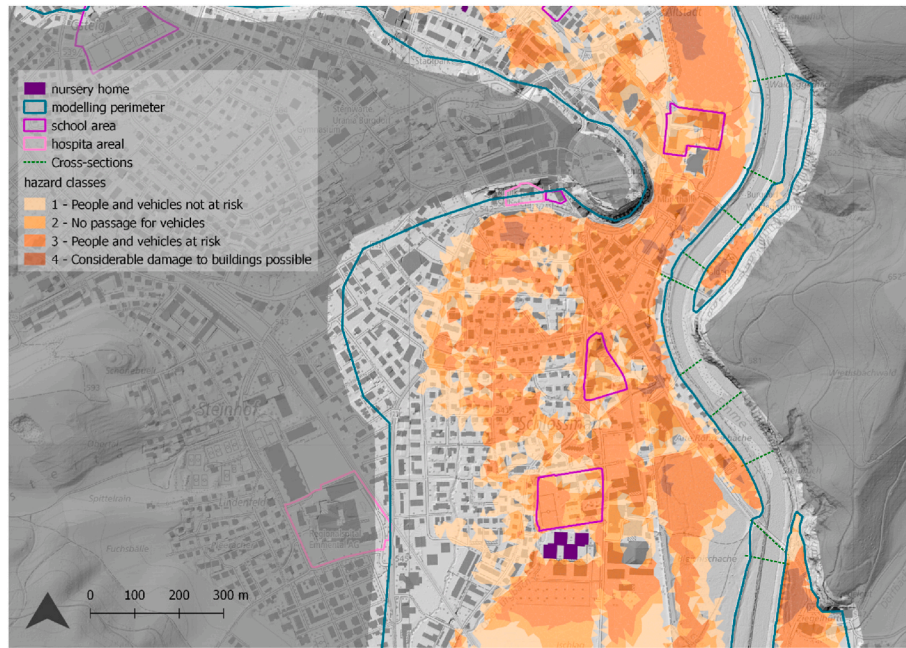
Fig. 9. Example of hazard map (from the surrogate model) of the Emme river near Burgdorf to support civil protection indicating predicted impact for people, vehicles and buildings and showing areas and buildings with vulnerable people (background swisstopo (2013; 2023) ).
