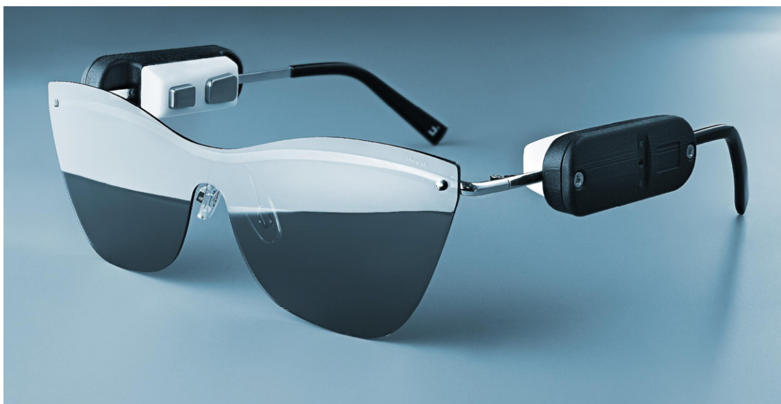
Figure 1. ULTEEM device consisting of sensors with active dry electrodes clipped onto the metallic frame of the eyeglasses.
