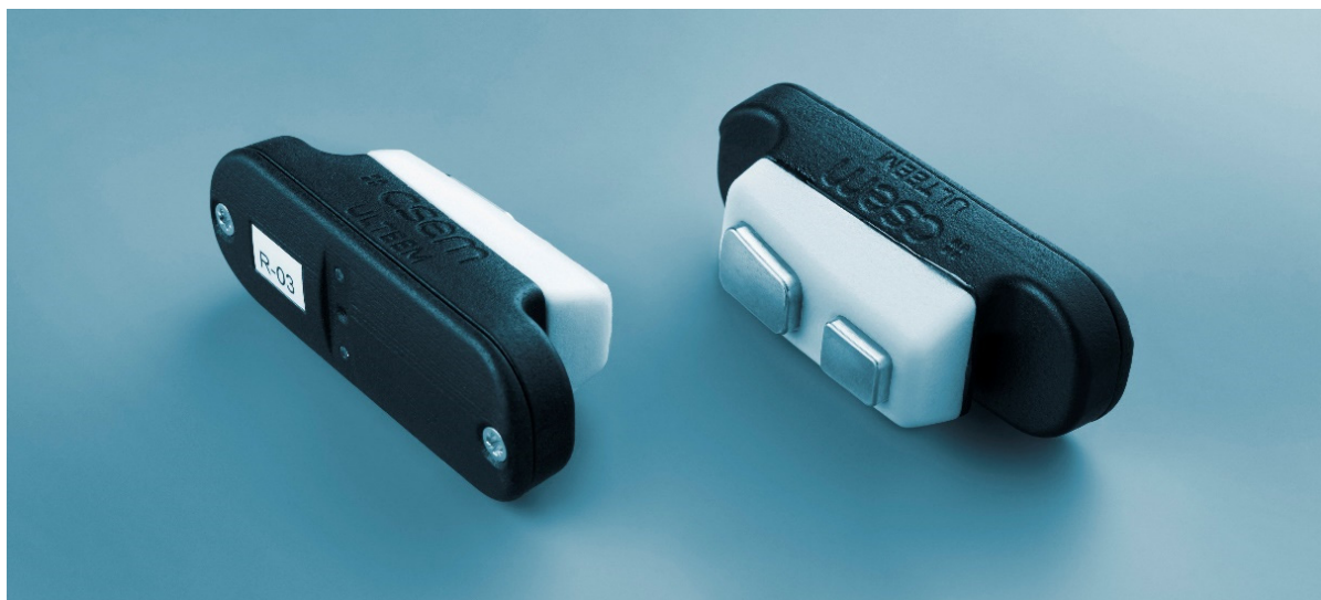
Figure 4. A close-up of a pair of ULTEEM clip-on sensors. The white part containing the stainless-steel dry electrodes and a spring backing is formed with a tapering to better adjust to the anatomy of an individual's temple.
