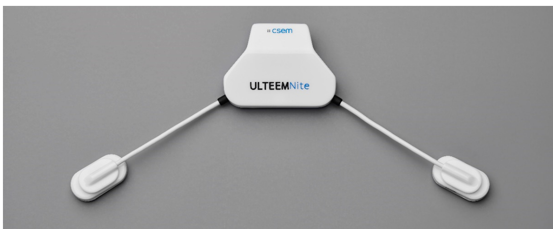
Figure 2. ULTEEMNite device with its central unit where processing, storage, and power management units are located, and the two sensor nodes equipped with active-dry electrodes.
