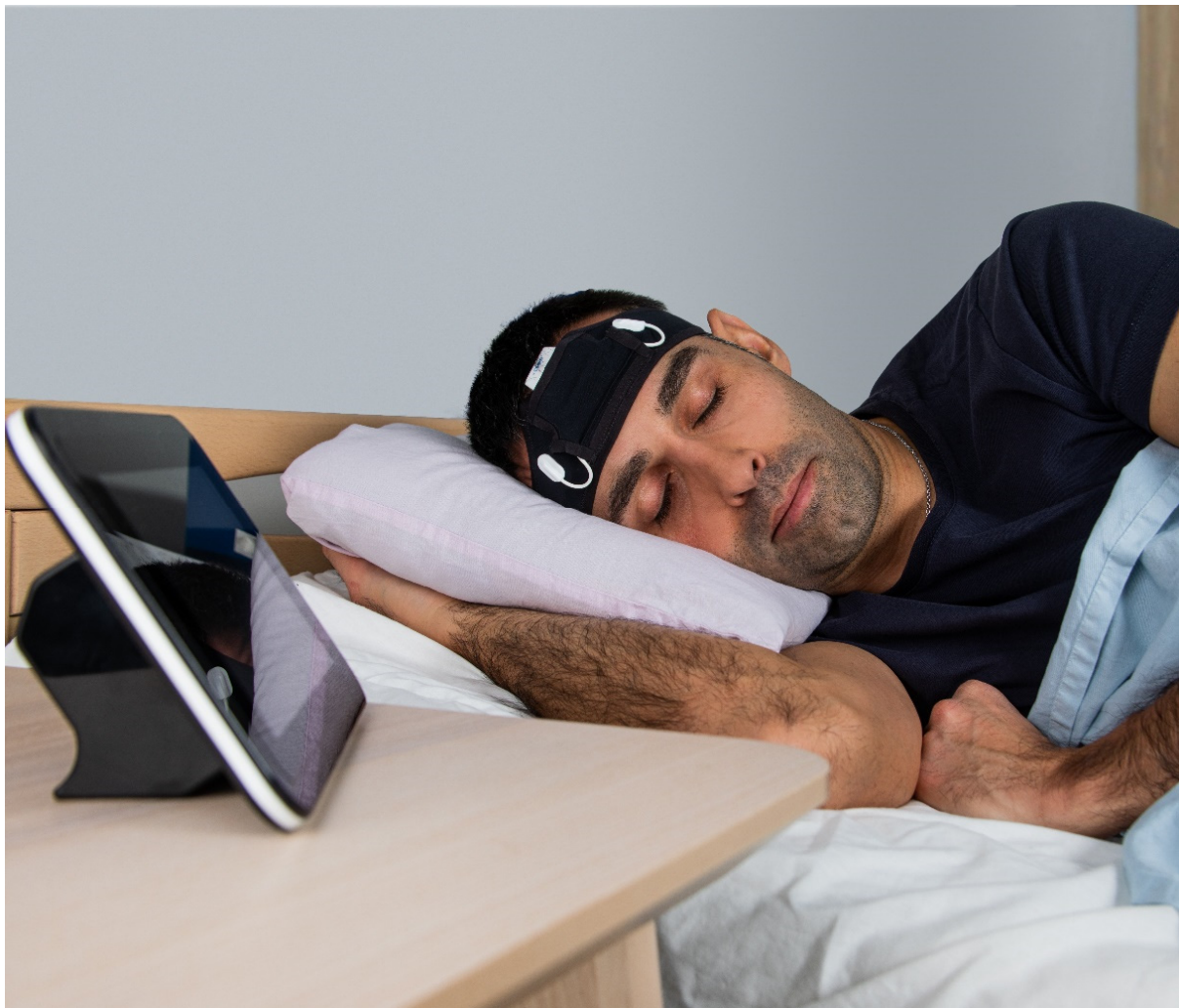
Figure 9. The ULTEEMNite system inserted into a headband and placed on the forehead. The central unit is slightly pulled out of its original place in the headbands pocket to increase its visibility. The device on the nightstand serves as a gateway to download recorded data from the ULTEEMNite device and to then upload it to a secure cloud server.
