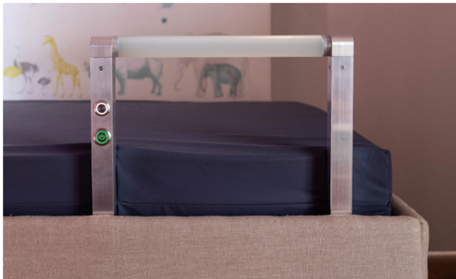
FIGURE 3 Smart Handle to turn bed on and off, illuminate the surrounding, and record bed and user movement, as well as day- and night-patterns.
