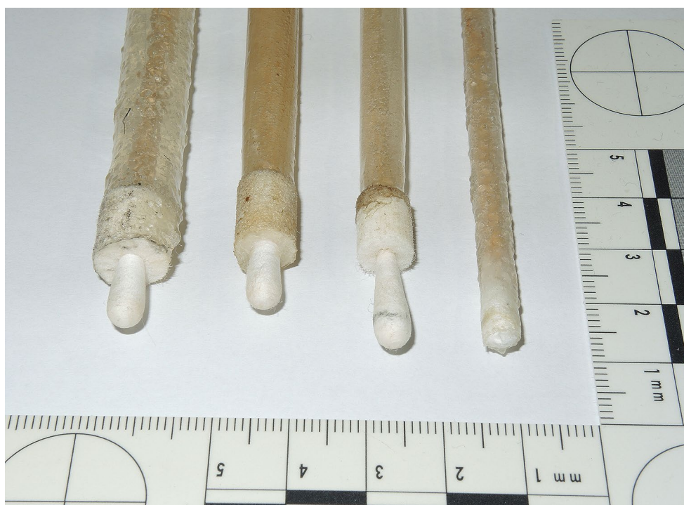
Fig. 1 Alginate-gelatine castings from cleaned revolver barrels, muzzle side on the left. From top: .38 special, 1.88 inch barrel (47.7 mm); .38 special, 4 inch barrel (100 mm); .357 Magnum, 6 inch barrel (150 mm)
