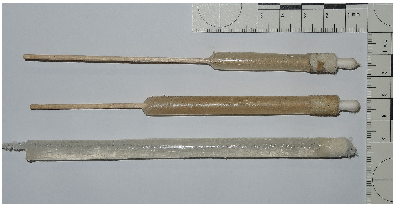
Fig. 1 Alginate-gelatine castings from cleaned revolver barrels, muzzle side on the left. From top: .38 special, 1.88 inch barrel (47.7 mm); .38 special, 4 inch barrel (100 mm); .357 Magnum, 6 inch barrel (150 mm)
