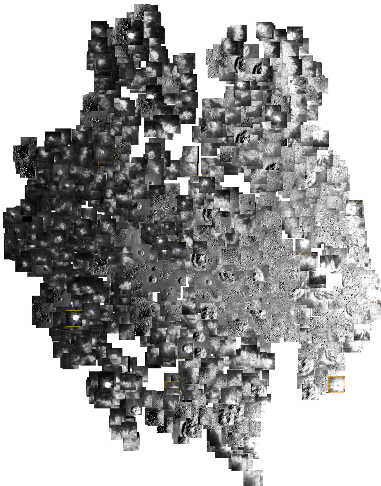
Fig. 8. t-SNE plot of top 2048 anomalous image patches from the crater test set. This type of t-SNE plot projects the high-dimensional structure between images into a 2-D representation seen here that can be both easily visualized while aiming to map images similar in high-dimensional space to nearby points in this 2-D visualization. Note that fresh craters can be larger than the model's 64 \times 64 pixel model window size, so that while each fresh crater only has one labeled positive sample, which is colored here, the same fresh crater may appear in multiple plotted samples, due to multiple, different model input windows covering the same fresh crater. Raw image credits to NASA/LROC/GSFC/ASU.
