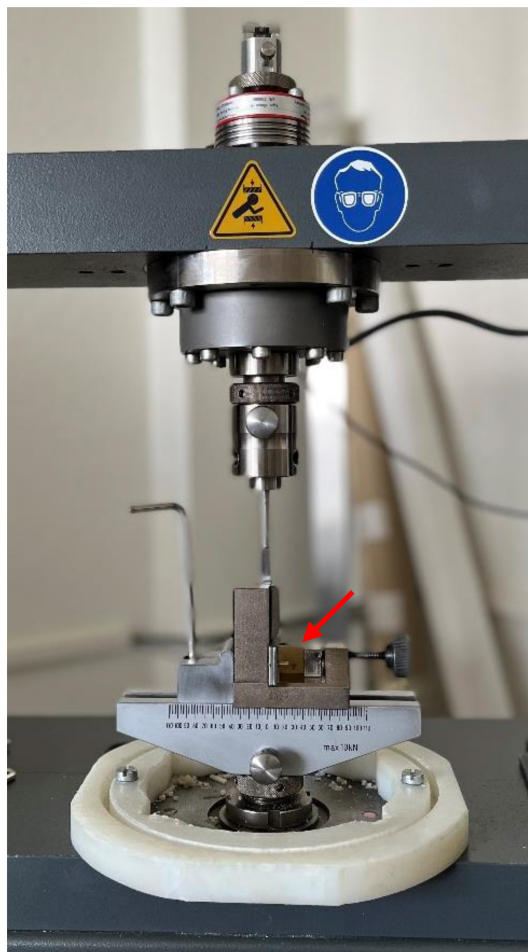
FIGURE 3. A specimen (arrow shows the acrylic embedding material) fixed during the shear bond testing using a universal testing machine.
