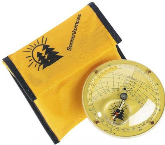
Fig. F.1. The sun compass (Sonnenkompass, Herzog Forsttechnik, Switzerland) used in the experiment. The perspex hemisphere displays the surrounding landscape on the plate, which allows to count the average daily number of sun hours for each month at the point it is placed.
