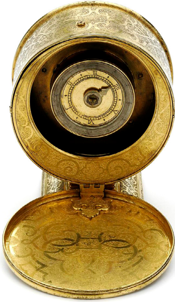
Fig. 8 Thomas Rückert, Waywiser, 1575, brass (cast, etched, gilded), iron, case: 11 cm (diameter) × 6.3 cm (depth), base: 7.1 cm (width) × 9.5 cm (depth), V 443 (photo: GRASSI Museum für Angewandte Kunst, Leipzig)
