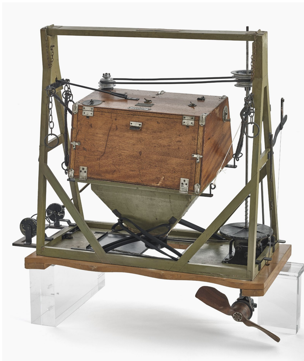
Fig. 1 Oskar Messter, film mapping camera Reihensbildner ("Rb I"), 1915, wood and metal, 890 × 860 × 400 mm. Munich, Deutsches Museum, Collection Photo- graphy-Cinematography, Inv. No. 56011 (56011_20220524_001_FotoraumSB_ND_ KRainer)
