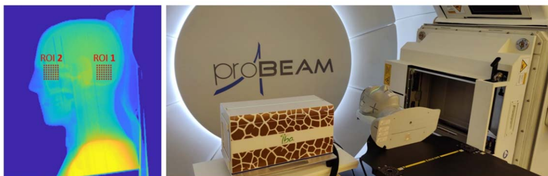
Figure 2. On the left: Position of the two ROI in the used head phantom. On the right: Experimental setup: the MLIC is positioned along the isocenter beam axis, on the distal end of the head phantom. The head phantom is placed AP on an immobilization pillow at the top of the couch. The gantry is positioned at 90^\circ .
