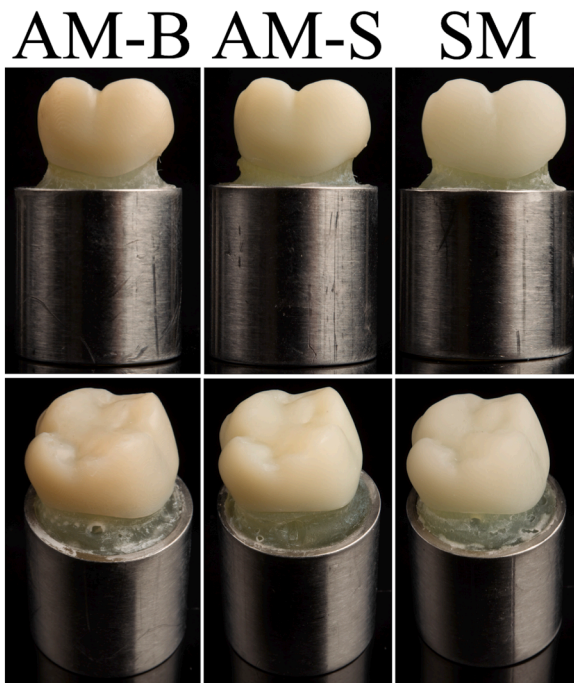
Fig. 1. Representative images of one crown from each material subgroup after cementation. AM-B; VarseoSmile Crown Plus. AM-S; Crowntec. SM; Vita Enamic.
